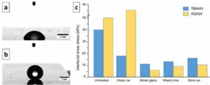
Figure 2: (a) Exemplification of the change in water contact angle on the reference (top) and DLIP-treated surface (bottom) for Ti6Al4V. (b) Ice adhesion of the laser-textured surfaces as measured by the interfacial shear stress under different atmospheric conditions for Ti6Al4V and Al2024 alloys.
