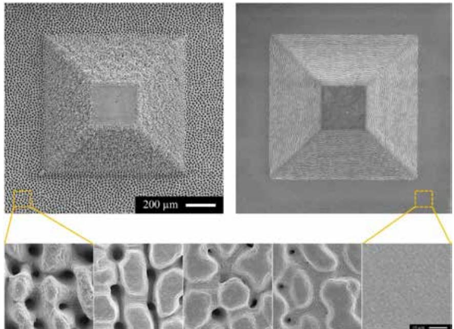
Figure 2: SEM collage of structures fabricated in stainless steel. From 6  $\mu\text{m}$  to 200 nm Sa surface roughness achieved. Results demonstrated by Fachgruppe Physik und Lasertechnik, Laserinstitut Hochschule Mittweida.
