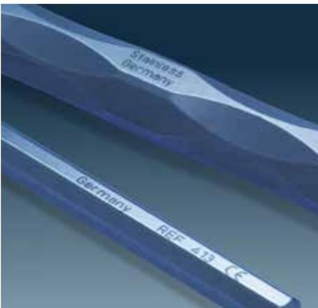
*Laser marking of steel medical instruments*
