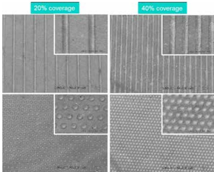
Figure 2: SEM images of laser textured cutting tools with 20% and 40% grooves and dimple density.
