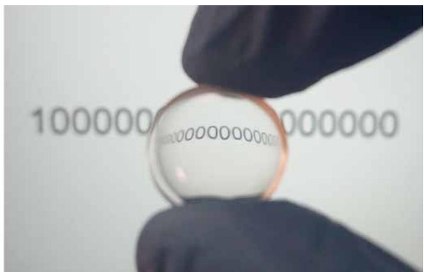
Figure 5: Polished curved surface processed with GHz burst.
