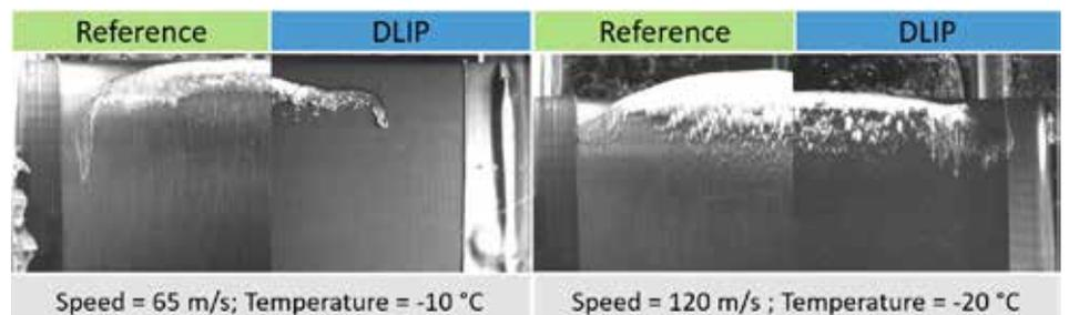
Figure 4: Comparison of the performance of unstructured and DLIP-treated Ti6Al4V airfoils in wind tunnel tests under different air speeds and air temperatures.
