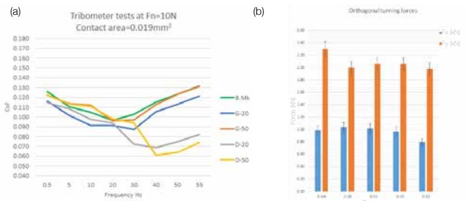
Figure 3: (a) Coefficient of friction as a function of sliding speed from tribometer tests and (b) cutting forces  $F_x$  and  $F_y$  from orthogonal turning tests for untextured and textured coated tool inserts [9].
