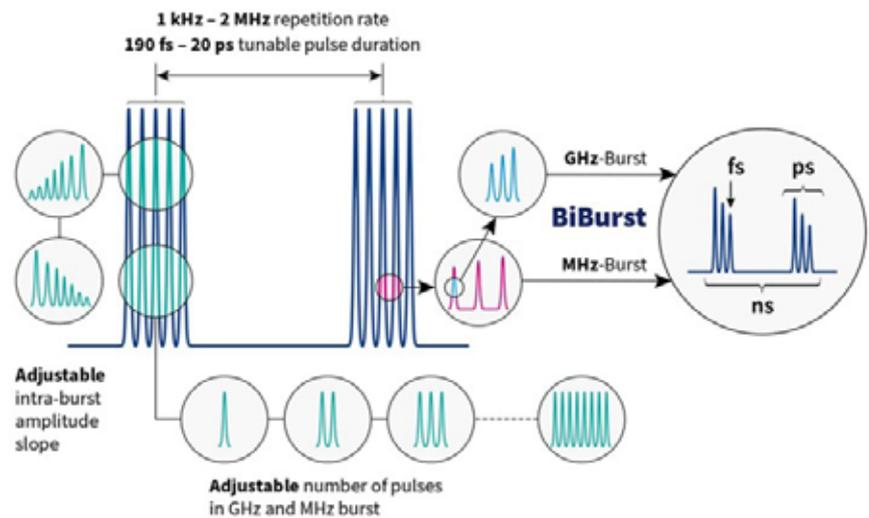
Figure 1: BiBurst - tunable GHz and MHz femtosecond burst scheme
