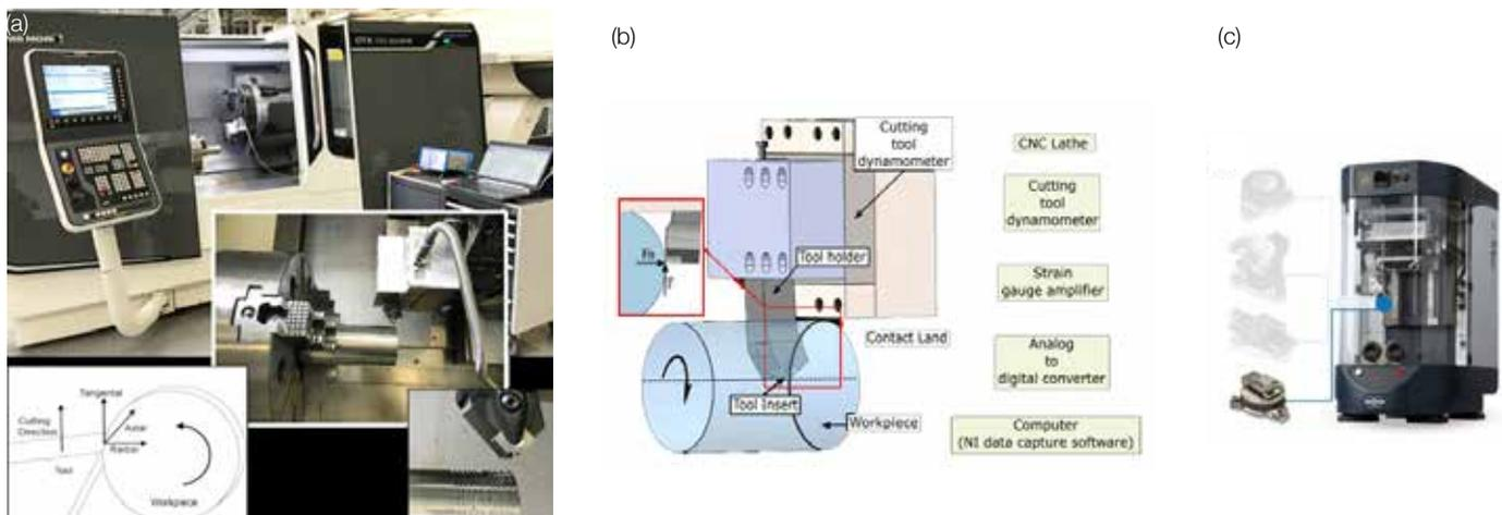
Figure 1: a) Orthogonal cutting test setup b) the data capture diagram and c) tribometer test setup.
