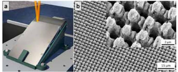
Figure 3: (a) Representation of the 3D processing of the NACA profile through DLIP and (b) resulting microstructures on the Ti6Al4V airfoil.
