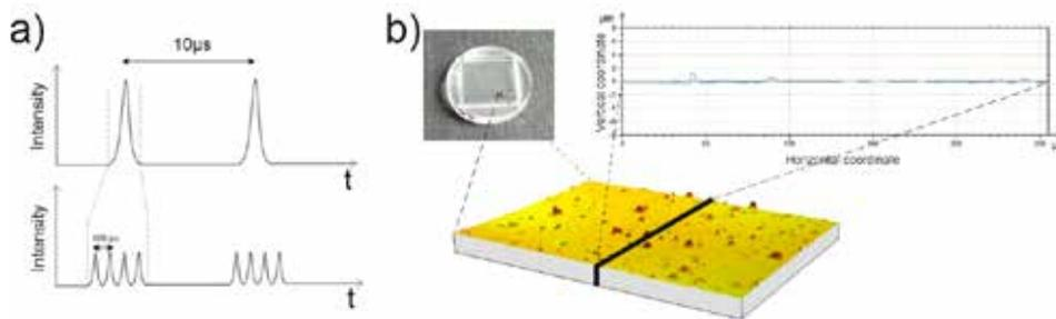
Figure 4: (a) Femtosecond laser pulse divided into bursts, (b) hydrophilic acrylic polymer after polishing parameters used: avg. power = 30 W, scanning velocity = 1 m/s, scanning pitch = 10 µm, number of GHz pulses = 10
