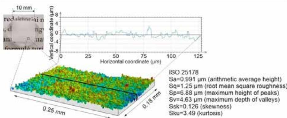
Figure 3: Hydrophilic acrylic polymer surface roughness after ablating using MHz
